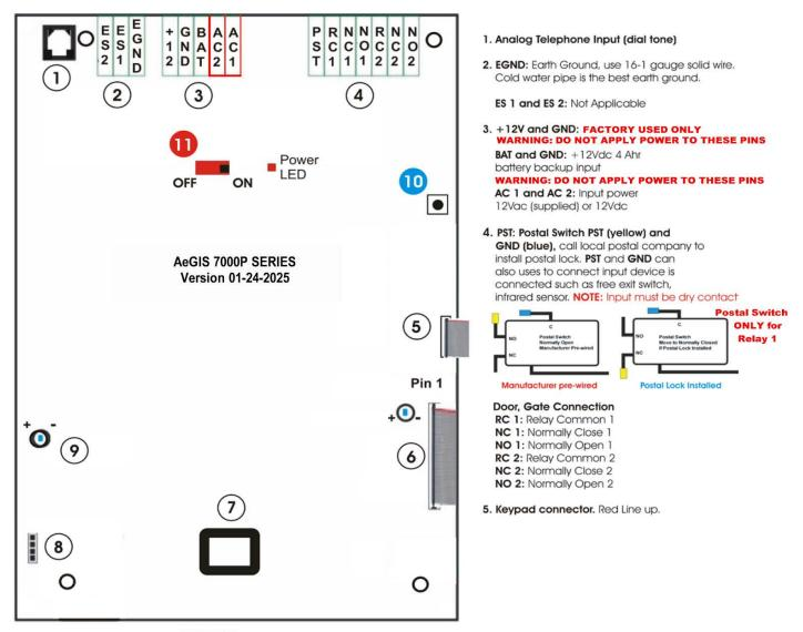
6. LCD Connector Red Line Up. WARNING: If you need to disconnect the LCD's ribbon cable, note down the direction and pins configuration. Connect the LCD's ribbon cable incorrectly, may damage the LCD or board. The RED LINE on the ribbon cable must be connected to pin 1.
